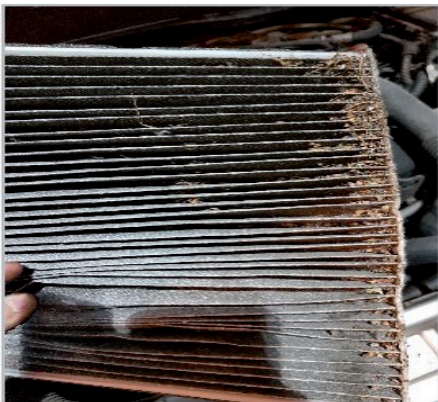
Photo 3 Contaminated cabin filter
