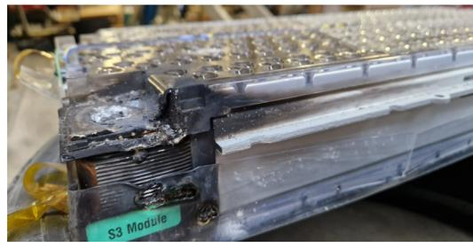
High temperatures can accelerate the degradation processes of electrode materials and electrolytes, leading to a reduction in battery capacity and life.
