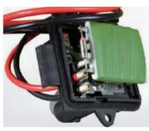
As for the high speed have a bypass connection (connected directly on the battery) this means no resistance but maximum power from the interior blower. The resistor is located inside the air flow from the blower motor, and this has an IMPORTANT effect on cooling down the resistor itself.
